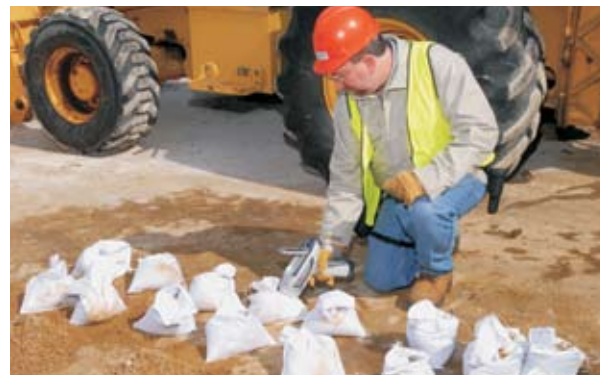
In-field instantaneous elemental analysis with the Thermo Scientific NITON XL3t.
