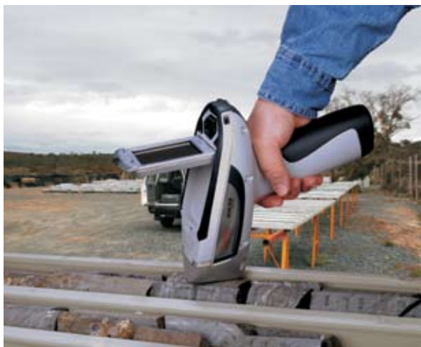
Direct analysis of core without requiring sample preparation.
