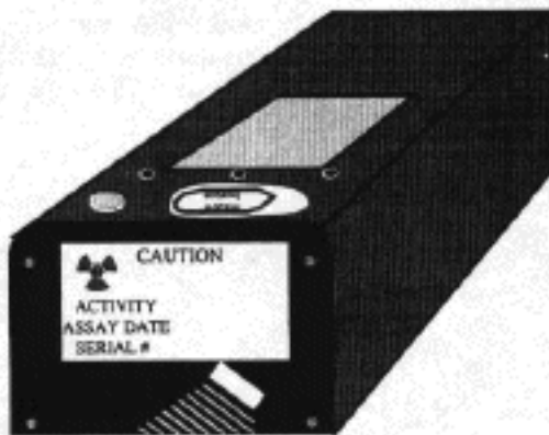
Fig. 5.06a Front/top view of XL showing the position of the inspection window and the source.
