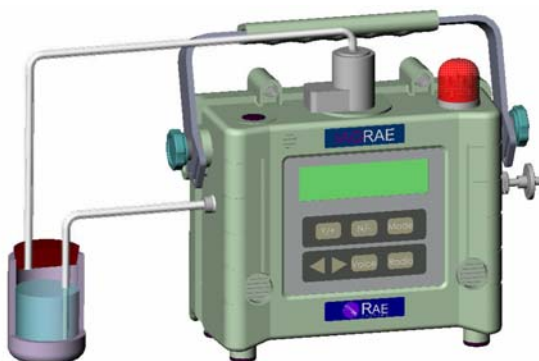
Figure 4-1 Water bubbler connections for span calibration
